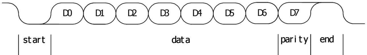
Picture 10 transmission sequence with parity bit (ASCII mode)
