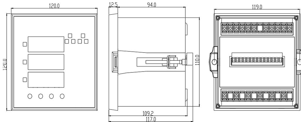
Picture 1 Installation Diagram
