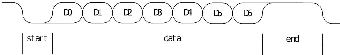
Picture 11 transmission sequence without parity bit (ASCII mode)
