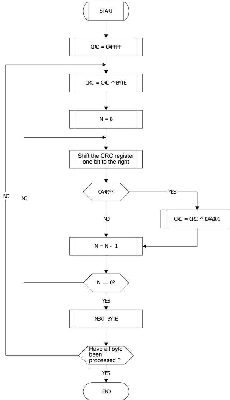
Picture 14, calculating progress of CRC-16 verify code
