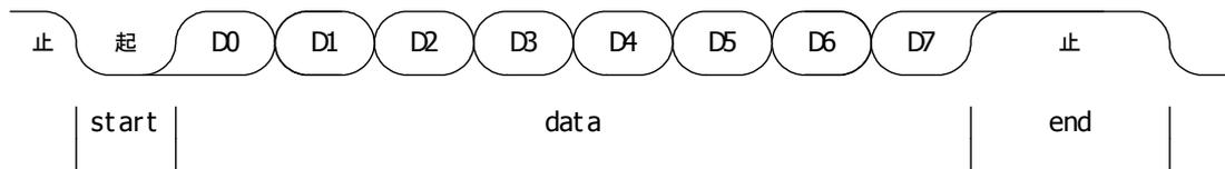
Picture 13 transmission sequence without parity bit (RTU mode)
