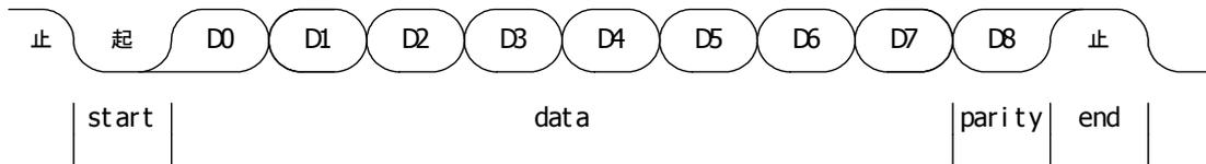
Picture 12 transmission sequence with parity bit (RTU mode)
