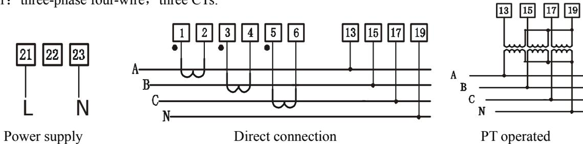
Picture 5 Wiring method
